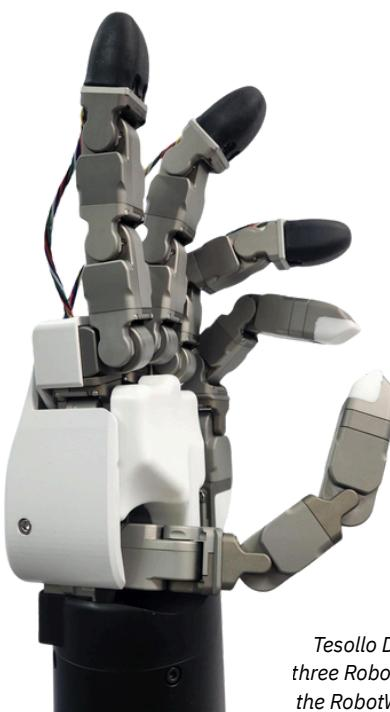
*Tesollo DG-5f gripper equipped with three RoboTact sensors as presented at the RobotWorld 2025 in Kintex, Korea.*
